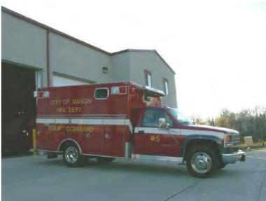
Squad 815 is a 1992 Chevrolet 3500 with an ambulance type box. This unit is used to haul specialty equipment such as Surface Ice Rescue, Hurst Extrication Equipment, and Confined Space Rescue Equipment. We also carry extra air cylinders to be used at fire incidents. This unit responds to every working fire with extra personnel, is used at the scene for firefighter rehab, and responds first to any vehicle pin in accident.
