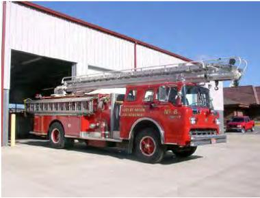
Ladder 818 is a 1973 Joyce on a Ford Chassis. This apparatus started out as an engine and in 1980 a 50 foot Snorkel was added. Ladder 818 has a 750 gallon per minute pump and carries 300 gallons of water. This is considered a reserve unit, but is still maintained and in service for response.
