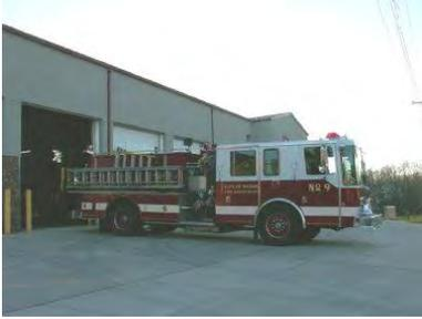
Engine 809 is a 1990 Grumman with a 1250 gallon per minute pump. This engine carries 1,000 gallons of water and 1,000 feet of large diameter supply line. This engine is the first out for any structure fire and vehicle fires during inclement weather. This engine has seating for 8 in an enclosed cab. This unit also carries some extrication equipment to respond to vehicle accidents.
