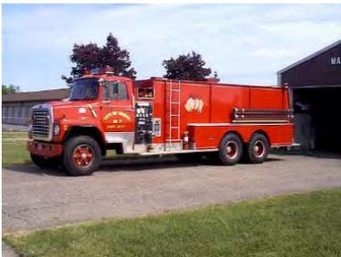
Tanker 807 is a 1984 3,000 gallon apparatus with a 500 gallon per minute pump on a Ford chassis. This tanker is housed at Station 2 on Curtis Street. It is the first tanker out when water is needed in the townships. This tanker is also part of the Ingham County Tanker Task Force and will go anywhere in Ingham County or the eastern part of Eaton County if needed.
