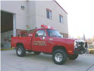
Brush 810 is a 1993 Dodge four wheel drive pick-up with a 100 gallon water tank and a 9 gallon per minute pump. This unit is used only for brush and wild land fires. Equipment carried includes portable water back packs, brooms, pitch forks, shovels, and a 5,000 lb winch and brush guard.
