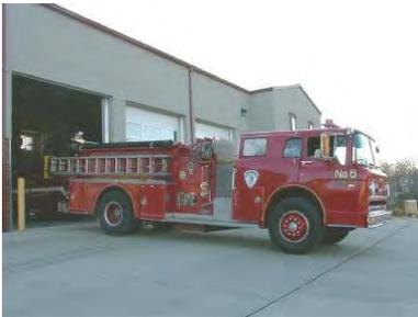
Engine 806 is a 1984 Grumman with a 1000 gallon per minute pump and a 1,000 gallon water tank. This engine is the first out for vehicle fires during good weather and third out for structure fires. We can carry 5 personnel, three in the open back and two in the cab.
