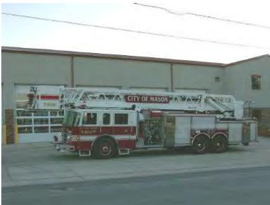
Tower 808 is a 2000 Pierce Dash 100 foot platform. It is powered by a 500hp Cummings diesel, with a 2000 gallon per minute pump. This unit is second out for any structure fires. It has an AMPS 10k hydraulic generator, 300 gallon water tank, a full compliment of ground ladders, and 1,000 feet of large diameter supply line. The cab will hold 6 personnel and has air supplied to the platform.
