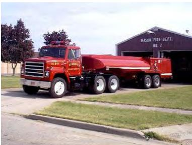
Tanker 811 is a 1983 International tractor with a 2,800 gallon 1947 water tank. It carries a 650 gallon per minute pump driven by its own diesel engine. There has been a lot of hard work done on this unit by our own members to make this a very dependable tanker. This is second tanker out for water supply in the townships.
