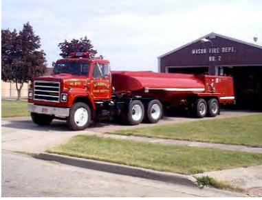
Tanker 811 is a 22 year old 1983 International tractor with a 2,800 gallon 58 year old 1947 water tank. It carries a 650 gallon per minute pump driven by its own diesel engine. There has been a lot of hard work done over the years to this unit by our own members to make this former government fuel hauler into a water tanker. This is second tanker out for water supply in the townships. This tanker is housed at Station 2 on Curtis Street.
