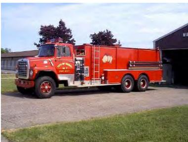
Tanker 807 is a 21 year old 1984 3,000 gallon apparatus with a 500 gallon per minute pump on a Ford chassis. This tanker is housed at Station 2 on Curtis Street. It is the first tanker out when water is needed in the townships. This tanker is part of the Ingham County Tanker Task Force and will travel anywhere in Ingham County or the eastern part of Eaton County if needed.
