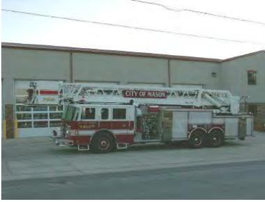
Tower 808 is a 4 year old 2001 Pierce Dash 100 foot platform. It is powered by a 500hp Cummings diesel, with a 2000 gallon per minute pump. This unit is first or second out for any structure fires. It has an AMPS 10k hydraulic generator, 300 gallon water tank, a full compliment of ground ladders, and 1,000 feet of large diameter supply line. The cab will hold 6 personnel and has air supplied to the platform.
