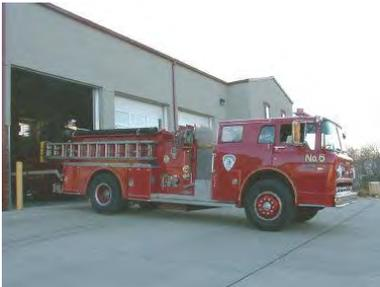
Engine 806 is a 21 year old 1984 Grumman with a 1000 gallon per minute pump and a 1,000 gallon water tank. This engine is the first out for vehicle and grass fires and third out for structure fires. We can carry 5 personnel, three in the open back and two in the cab.
