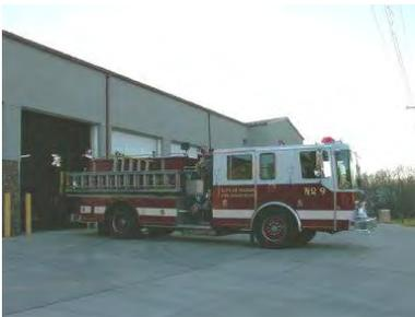
Engine 809 is a 15 year old 1990 Grumman with a 1250 gallon per minute pump. This engine carries 1,000 gallons of water and 1,000 feet of large diameter supply line. This engine is the first or second out for any structure fire and vehicle fires during inclement weather. This engine has seating for 8 personnel in an enclosed cab. This unit also carries some extrication equipment to respond to vehicle accidents.
