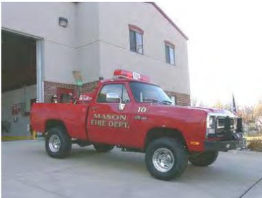
Brush 810 is a 12 year old 1993 Dodge four wheel drive pick-up with a 100 gallon water tank and a 9 gallon per minute pump. This unit is primarily used for brush/ wild land fires, and occasionally to transport personnel. Equipment carried includes portable water back packs, brooms, pitch forks, shovels, and a 5,000 lb winch and brush guard.
