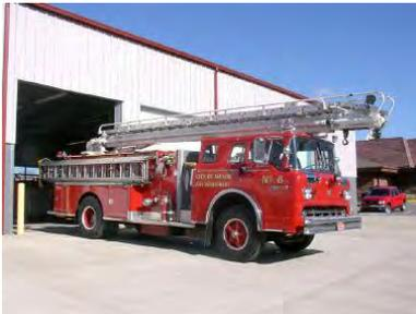
Ladder 818 is a 32 year old 1973 Joyce on a Ford Chassis. This apparatus started out as an engine and in 1980 a 50 foot Snorkel was added. Ladder 818 has a 750 gallon per minute pump and carries 300 gallons of water. This is considered a reserve unit, but is still maintained and in service for response.
