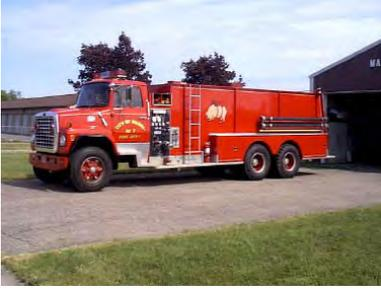
Tanker 807 is a 22 year old 1984 3,000 gallon apparatus with a 500 gallon per minute pump on a Ford chassis. This tanker is housed at Station 2 on Curtis Street. It is the first tanker out when water is needed in the townships. This tanker is part of the Ingham County Tanker Task Force and will travel anywhere in Ingham County or the eastern part of Eaton County if needed.
