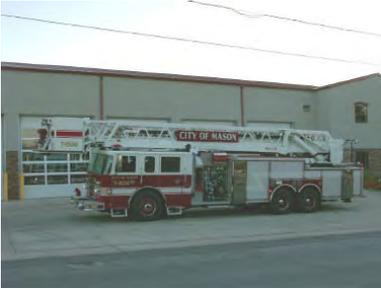
Tower 808 is a 5 year old 2001 Pierce Dash 100 foot platform. It is powered by a 500hp Cummings diesel, with a 2000 gallon per minute pump. This unit is first or second out for any structure fires. It has an AMPS 10k hydraulic generator, 300 gallon water tank, a full compliment of ground ladders, and 1,000 feet of large diameter supply line. The cab will hold 6 personnel and has air supplied to the platform.
