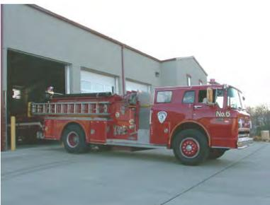
Engine 806 is a 22 year old 1984 Grumman with a 1000 gallon per minute pump and a 1,000 gallon water tank. This engine is the first out for vehicle and grass fires and third out for structure fires. We can carry 5 personnel, three in the open back and two in the cab.
