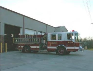
Engine 809 is a 16 year old 1990 Grumman with a 1250 gallon per minute pump. This engine carries 1,000 gallons of water and 1,000 feet of large diameter supply line. This engine is the first or second out for any structure fire and vehicle fires during inclement weather. This engine has seating for 8 personnel in an enclosed cab. This unit also carries some extrication equipment to respond to vehicle accidents.
