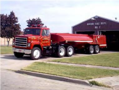
Tanker 811 is a 23 year old 1983 International tractor with a 2,800 gallon 58 year old 1947 water tank. It carries a 650 gallon per minute pump driven by its own diesel engine. There has been a lot of hard work done over the years to this unit by our own members to make this former government fuel hauler into a water tanker. This is second tanker out for water supply in the townships. This tanker is housed at Station 2 on Curtis Street.
