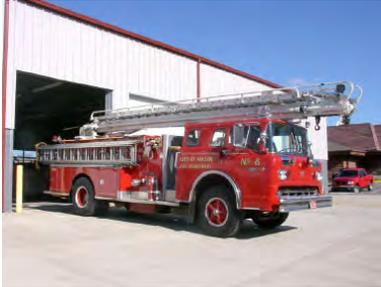
This 1973 apparatus has been in a reserved status since delivery of Tower 808 and has seen little use. A hydraulic leak in the cylinder that extends the ladder was discovered in October. After contacting the repair company it was found that repairs would cost between \$2,500 and \$8,000 depending on the severity of work necessary. It was decided that in the best interest of the City not to expend more money into this apparatus.
