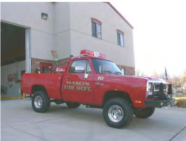
Brush 810 is a 13 year old 1993 Dodge four wheel drive pick-up with a 100 gallon water tank and a 9 gallon per minute pump. This unit is primarily used for brush/ wild land fires, and occasionally to transport personnel. Equipment carried includes portable water back packs, brooms, pitch forks, shovels, and a 5,000 lb winch and brush guard.
